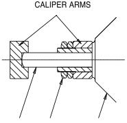
PUSHROD LOCKNUTS THRUSTER
