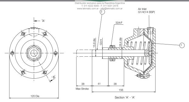
This range of pneumatically operated brakes uses dry and filtered compressed air at pressures up of 7 bar. Pneumatic brakes require a control valve which may be operated either manually, or by pneumatic or electrical signal.
